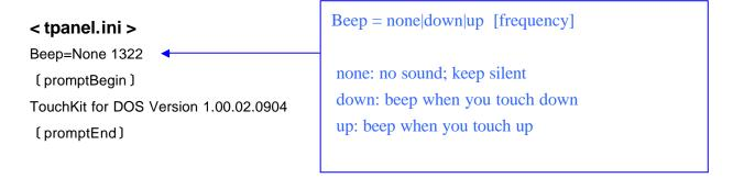
After saving new **tpanel.ini**, users can force the driver to reload the new **tpanel.ini** by executing **C:\TouchKit\>tpanel -r** Other adjustment can be checked by **C:\TouchKit\> tpanel -?**
